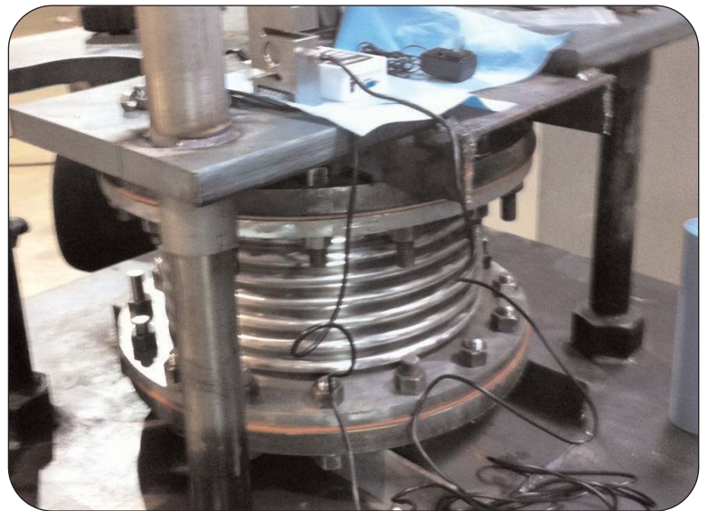
Thorburn's Model RLB-SF Cyclic Movement Testing
